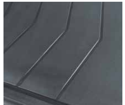
Bed surface features grooves for fluid management
