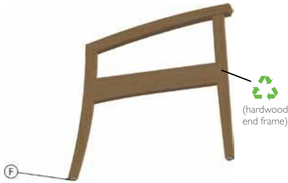
F: Using pliers, remove the two glides from each end frame.
